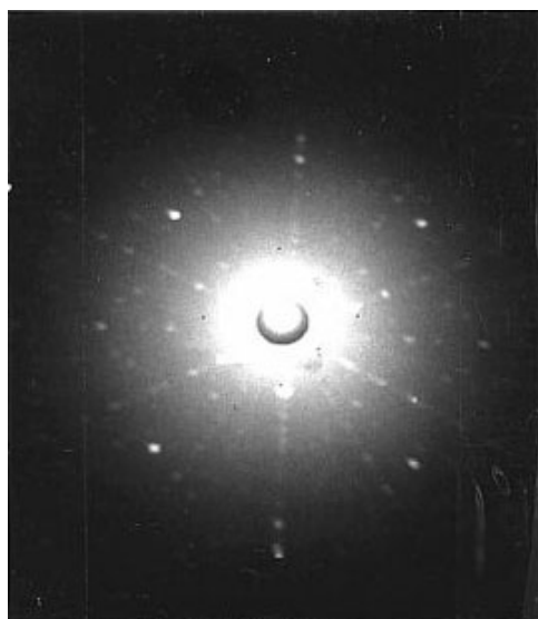
Figure 2. X-ray Laue back-reflection photograph of a crystal of \text{Co}_3\text{V}_2\text{O}_8 showing the (100) orientation.
